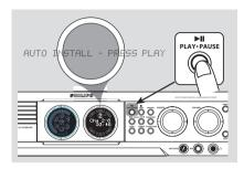
Connect the system to the power supply, "AUTO INSTALL - PRESS PLAY" appears. OR
